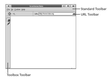
**FIGURE 5.4**Three types of toolbars are created by KCustomActions.
